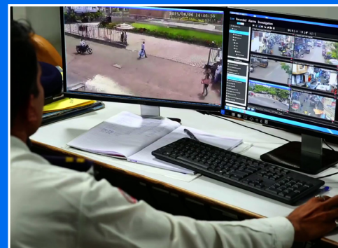
PCS operators receive real-time automatic alerts of events of interest such as security breaches, loitering, crowding, and unattended objects.
