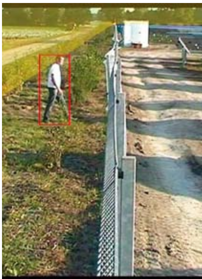
▲ Analytics can be deployed at perimeters, to detect unauthorized intrusion. (Image courtesy of Viasys Intelligent Video)
