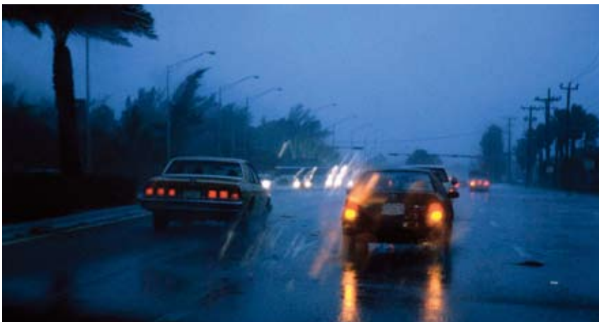
▲ Headlights of a moving vehicle, coupled with the speed of movement, and the size and shape of shadows can be similar to a person or a group of people. This makes it difficult for analytics to make a distinction.
